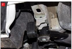
Once happy with fitment of Scorpion Exhaust, fully tighten up all clamps and fixing and plug in the electronic valve motors.
